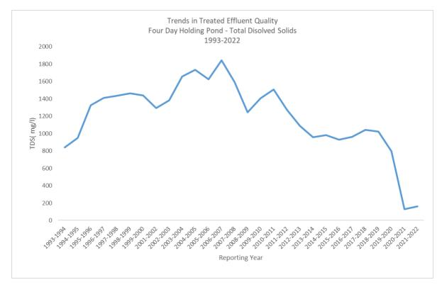
FIGURE 17. Trends in Treated Effluent Quality from the Four Day Holding Pond - TDS
