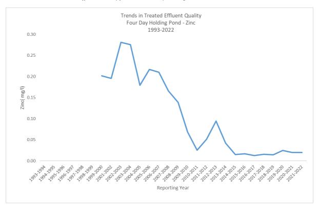
FIGURE 19. Trends in Treated Effluent Quality from the Four Day Holding Pond – Zinc
