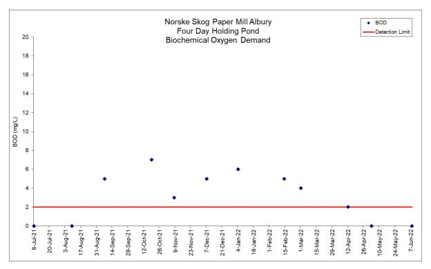
FIGURE 6. Biological Oxygen Demand of Treated Effluent from the Four Day Holding
